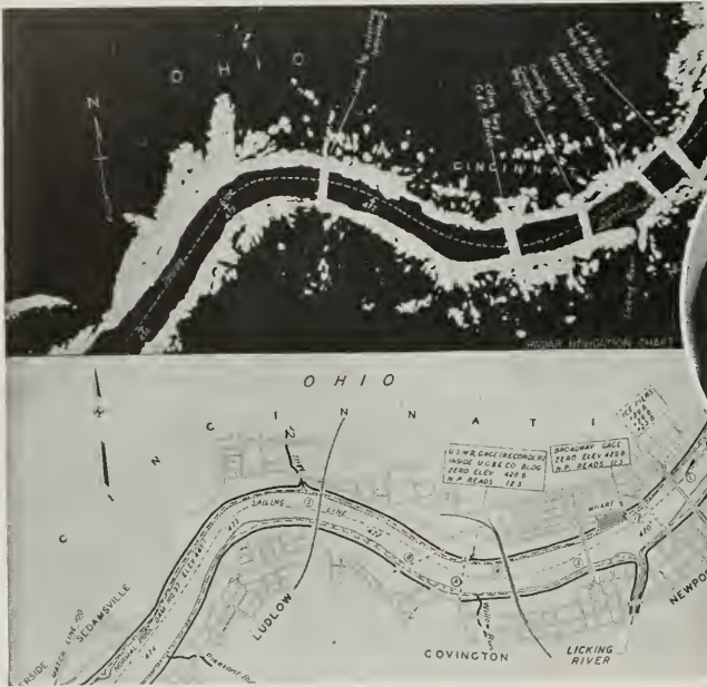
COMPARISON OF RADAR MOSAIC (TOP) WITH STANDARD CHART OF SAME SECTION OF RIVER SHOWS ACCURACY OF NEW MAPPING METHOD.
